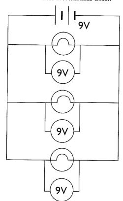
▲ In a parallel circuit, the voltage across each component represents the entire supply voltage of the battery.
