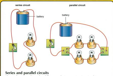
These diagrams show the differences between circuits wired in series and those wired in parallel.
